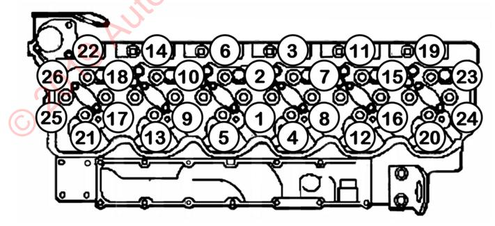
Note: It will be necessary to machine the lower rocker arm cover at the No. 24 bolt hole location in the torque sequence to facilitate installation of the lower rocker arm cover (see illustrations).
