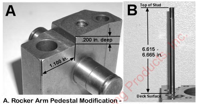
It will be necessary to mill a step in all six pedestals to the specified amount. The step must be parallel (+/-.005 in.) with the bottom of each rocker arm pedestal.
